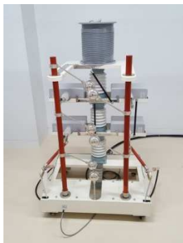
Impulse Voltage Generator
