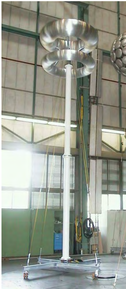
2400 kV impulse voltage divider
