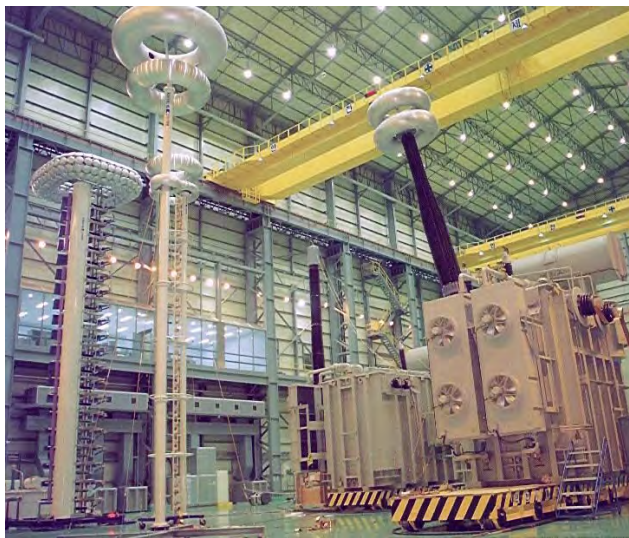
Impulse test system with 4000 kV impulse generator & divider and 3600 kV multiple chopping gap
