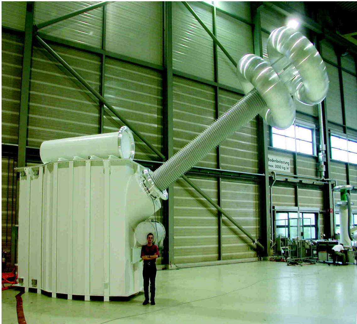
Tank type test transformer 750 kV, 2100 kVA
