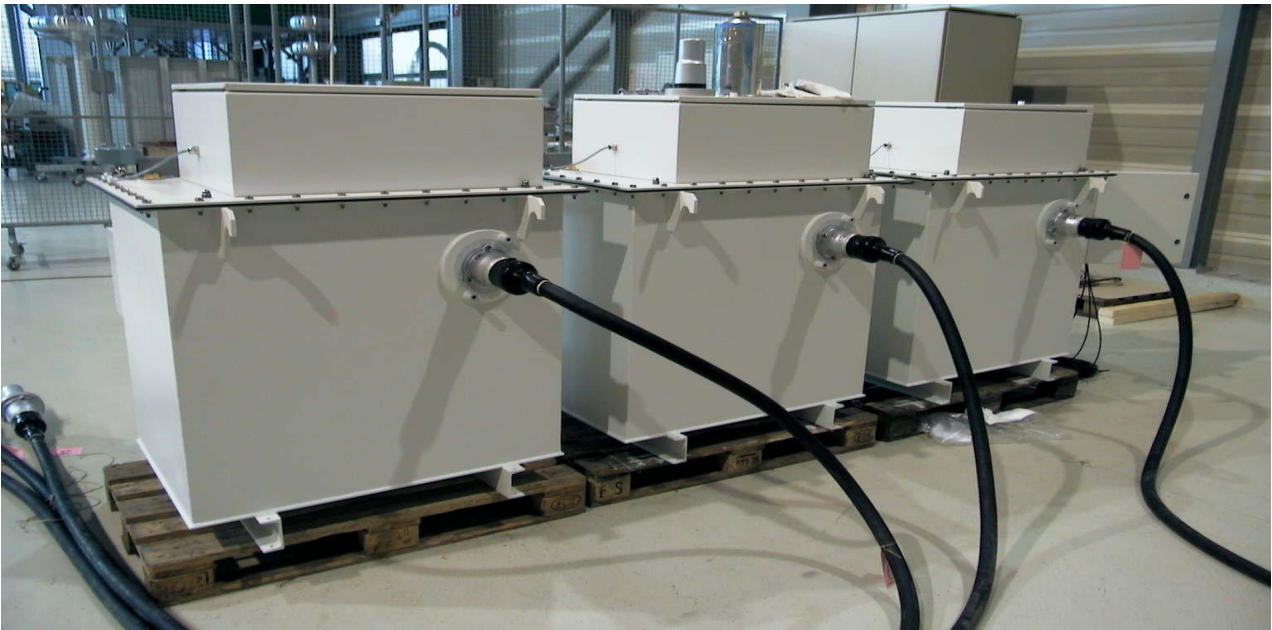
Example of a 3 phase 70 kV test system with MV cable connectors and leads
