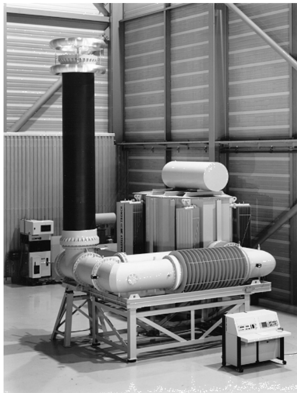
Example of a 700 kV, 2'100 kVA system with SF 6 bus comprising damping resistor, coupling capacitor & SF 6 - air bushing
