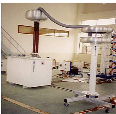
250 kV, 50 kVA test transformer and HV divider
